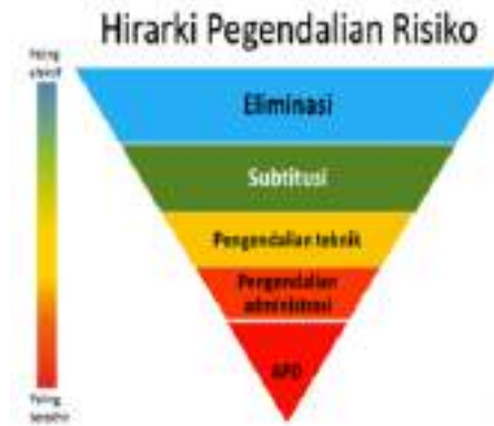
Gambar 5.2: Hierarki Pengendalian Risiko K3 dari NIOSH (National Institute For Occupational Safety and Health) (Kemenkes RI, 2018)
